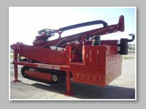
The GP-600 is part of the Geo-Swing family. With its compact size of only 6.8 ft by 16 ft, it is one of the most versatile track mounted rigs in the geothermal market. The rig is mounted on a turret style track system, which allows drilling and maneuverability in confined spaces without leaving a heavy footprint.
